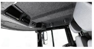
A long roof protects the user from direct sunlight regardless of the large window areas. User comfort is further boosted by bottle storage, in-cabin smartphone charging and plenty of storage space for documents and tools.
